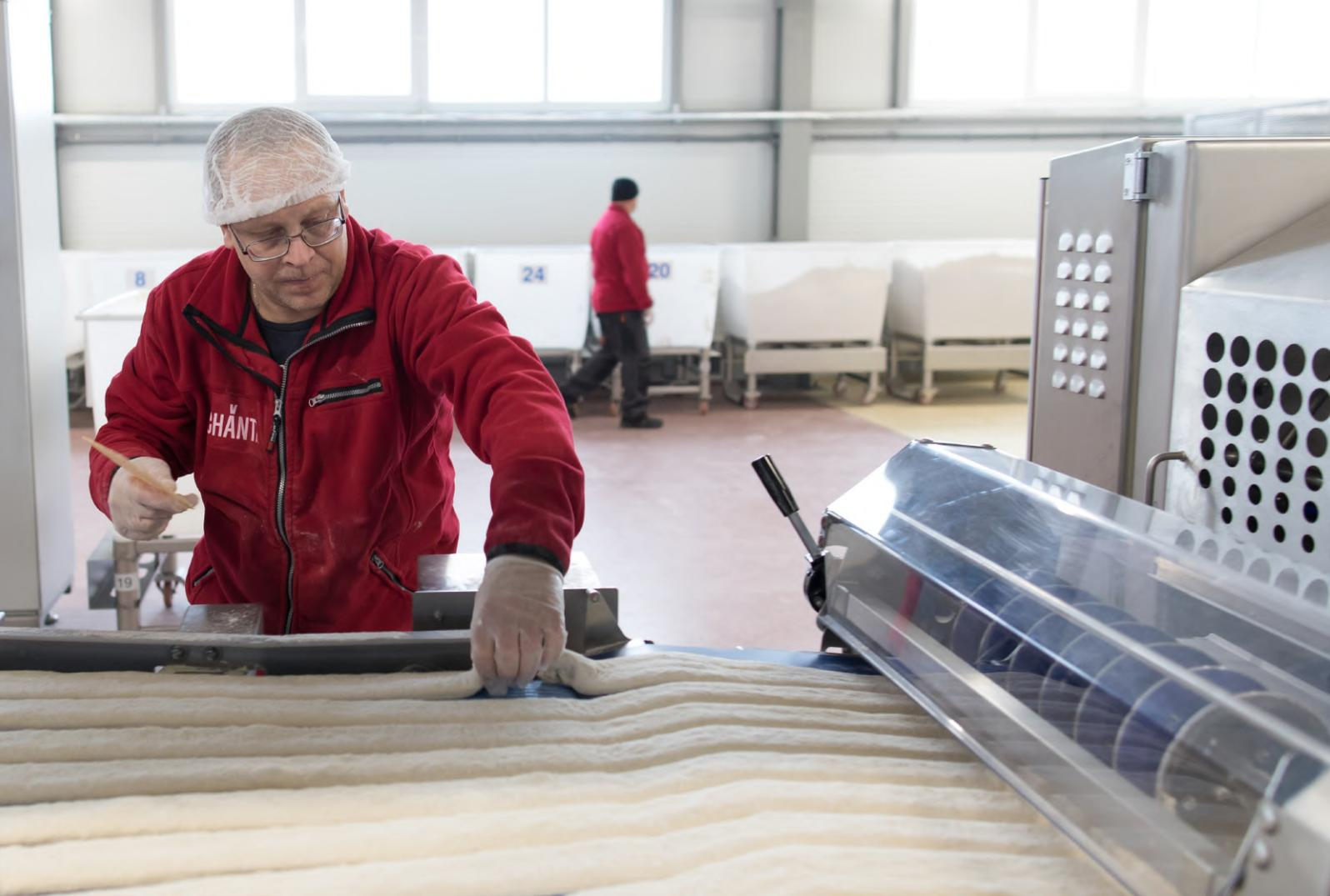
To maintain the structure of the dough, a German **automated line** was installed **for working with soft dough types**. Unlike traditional dough machines with stressful mechanical dough processing, we use a soft stress-free dough handling system.
