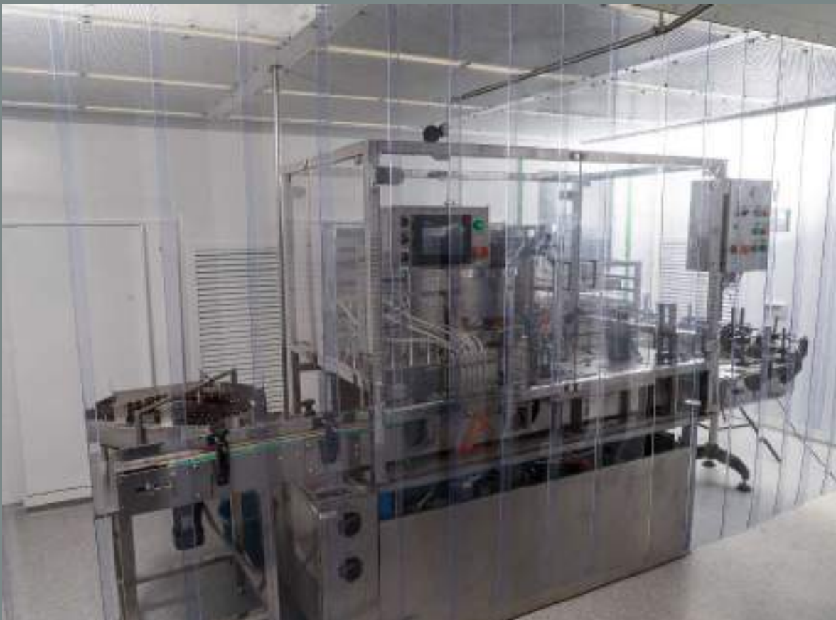
Line for bottling liquid dosage forms and other non-toxic aqueous solutions in plastic containers of 100-200 ml. Project capacity (annual) - 2 million bottles
