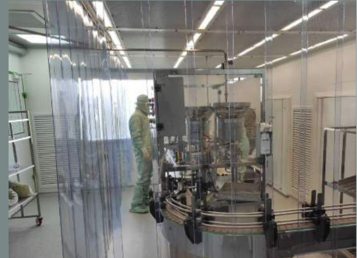
Line for bottling liquid dosage forms and other non-toxic aqueous solutions in plastic containers of 100-200 ml. Project capacity (annual) - 2 million bottles
